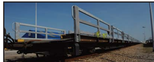
A shuttle without pagodas which will soon be used to make operations easier and give a new outlook to cross-Channel rail freight
