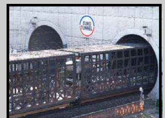
The first trucks destroyed by the fire, possibly where the disaster struck. The wagons are not deformed.
