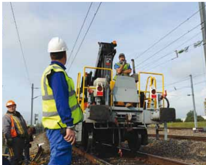
Seven Eurotunnel works train wagons are now equipped with electric motors.
